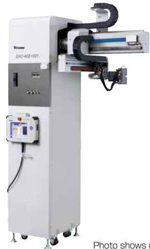
Photo shows robot with optional suction EOAT
